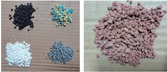
a: 4 种近似球形颗粒肥料 a: Four types of approximately spherical granular fertilizers b: 不规则氯化钾颗粒 b: Irregular potassium chloride particles
